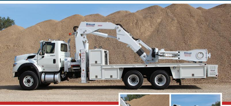
The Stellar 28000 OTR series tire service crane fits the need of OTR tire service technicians who need something that can handle it all. A 320-degree turntable rotation system driven by a worm gear / pinion system ensures rock solid performance. This crane features a lifting capacity of 28,000 lbs. at 10' and 17,200 lbs. at 16'3" of total reach, without the tire manipulator.
